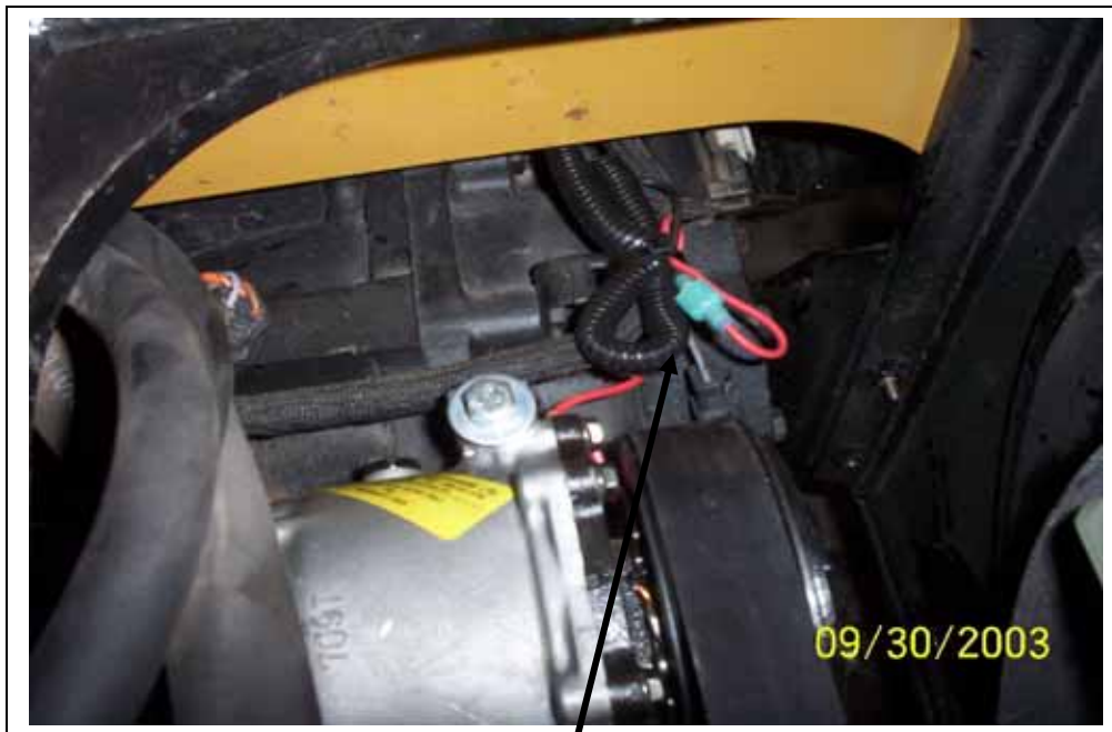
Connect the clutch wire to the wire on the compressor.
