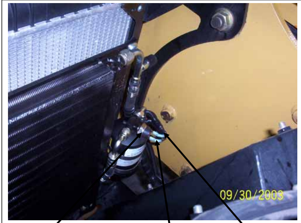
Binary switch on drier.
