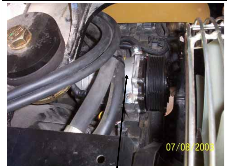
Compressor bolted into place
