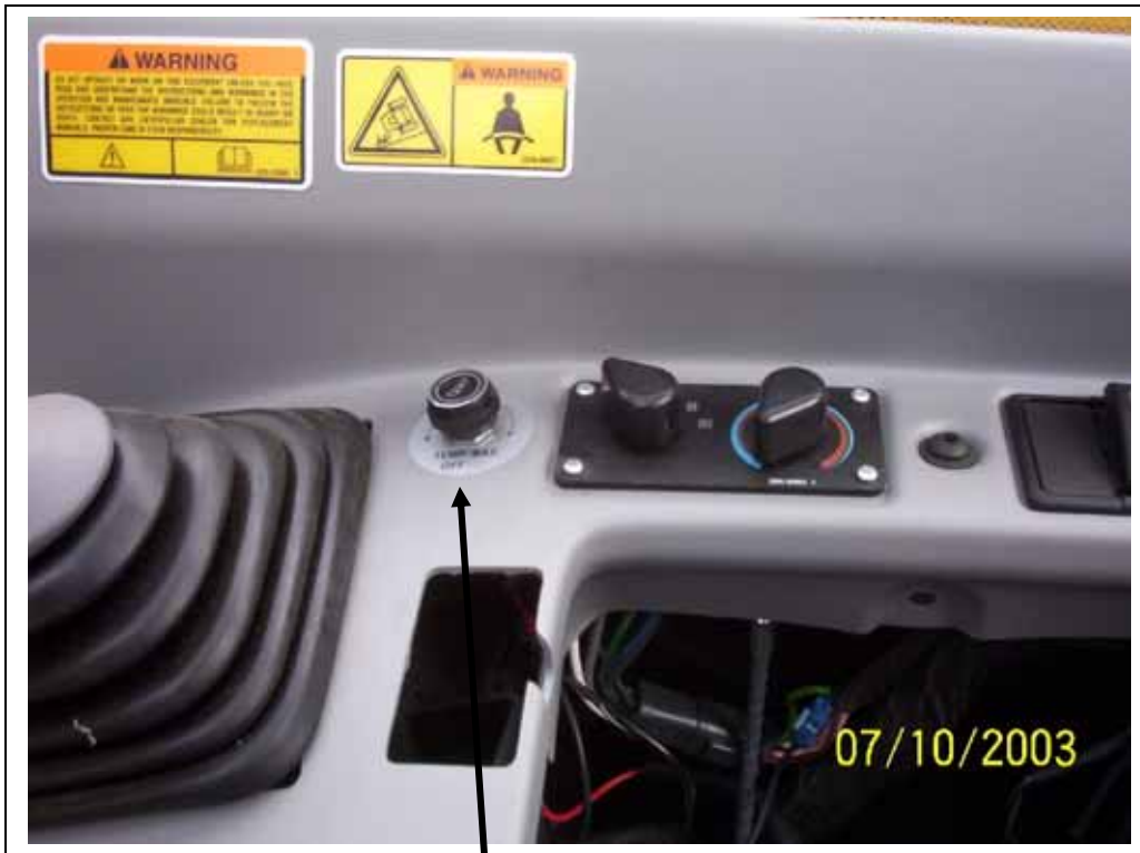
Thermostat, decal and knob in place. Test for full 12Volt power to the thermostat on all three blower speeds.
