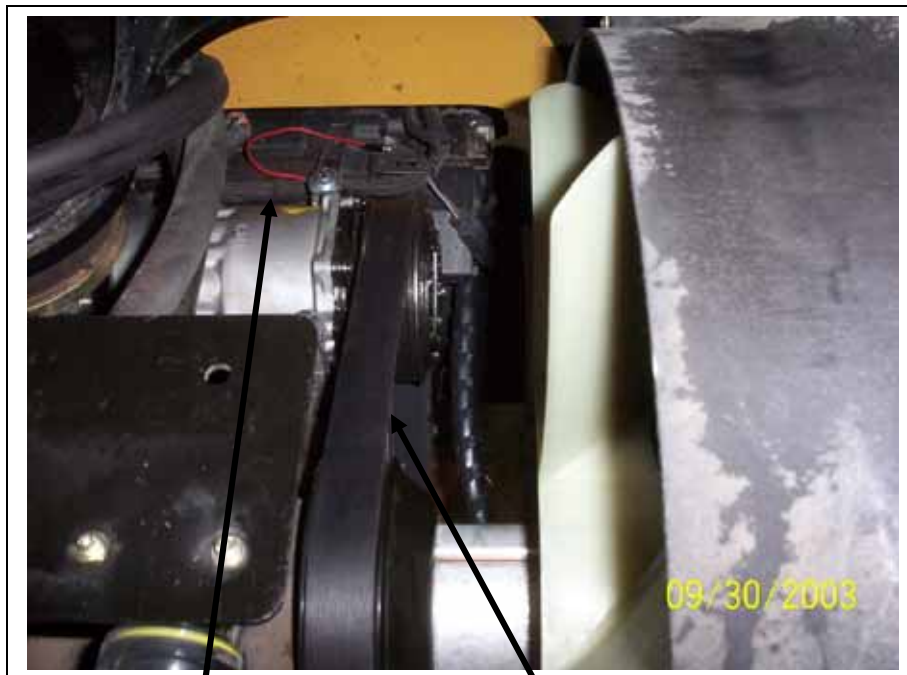
Oil fill plug and clutch wire point towards the cab.
