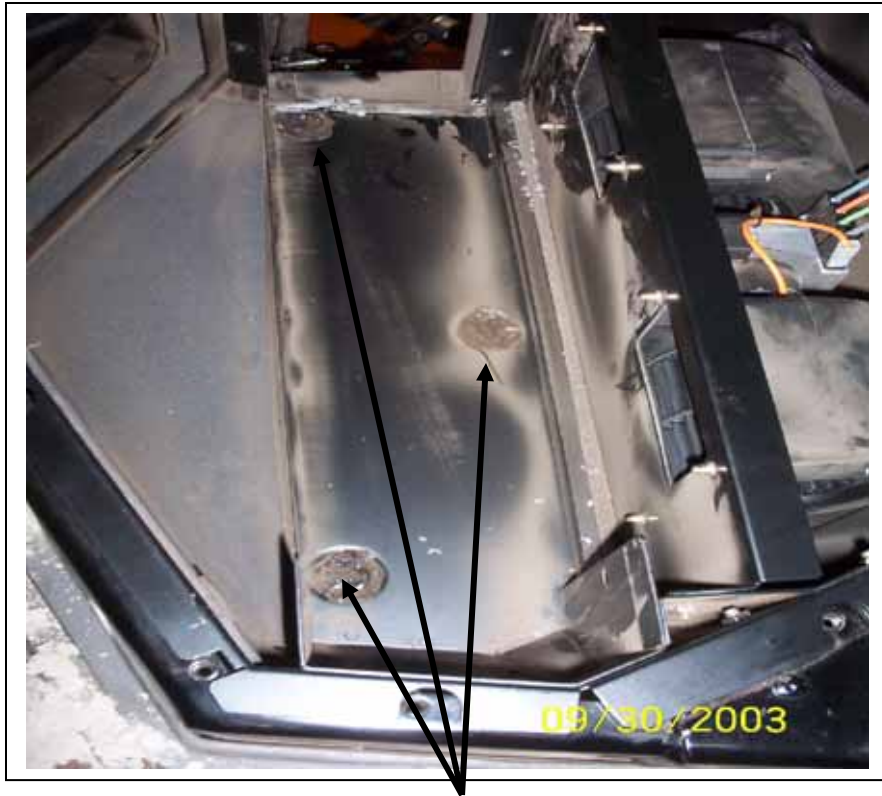
Remove the three plugs in the bottom of the box to accommodate the drain tubes.
